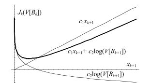
Fig. 3. A schematic illustration of the cost function of an additional experiment at time k. The value of the control is optimized to support a single step look-ahead DP algorithm.
